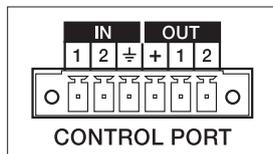
The CONTROL PORT offers two freely programmable control inputs and control outputs as well as the reference connections for ground potential and +5V. Using the PC Windows software IRIS, the control inputs can be configured and serve for instance for Power-On / Stand-by switching, preset switching or parameter control.
